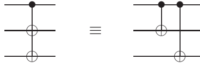
Figure 4.13. Controlled-NOT gate with multiple targets.
